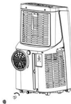
To empty the container, switch off the appliance and remove the plug from the socket. Place the end of the drain over a container to collect the condensate, undo the ring-nut by turning it anticlockwise, and remove the plug of the bottom drainage hole.
